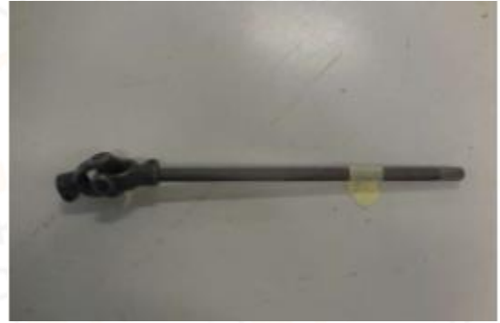
The removed shaft with U-joint.
