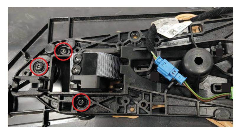
Feed the strap through the faceplate and back through the other side as shown. The faceplate should be loose and will be tightened later.
