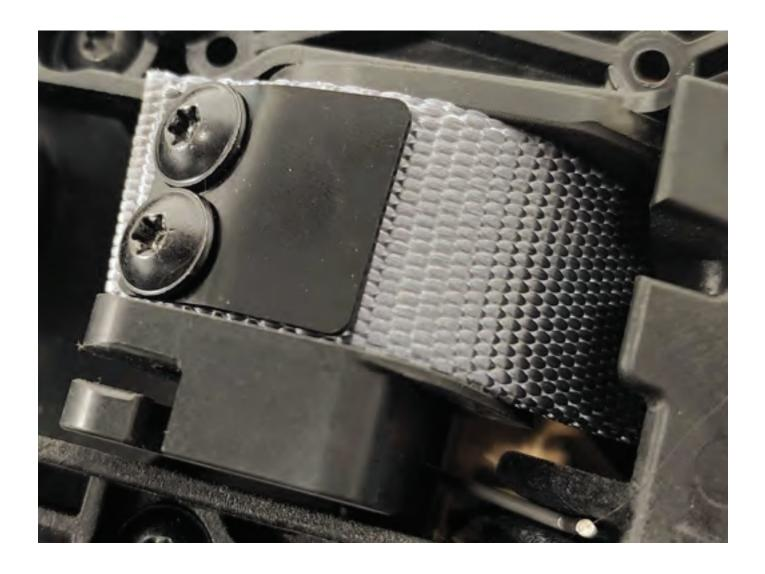
Feed the strap through the part as shown and reinstall the retaining frame back to the door. Reinstall the 3 TORX screws from the original retainer back in the locations shown.
