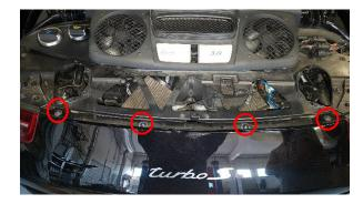
Loosen 2x Torx T25 and gently pull the rear light straight back. Disconnect the cable connector. Do this on both sides.
