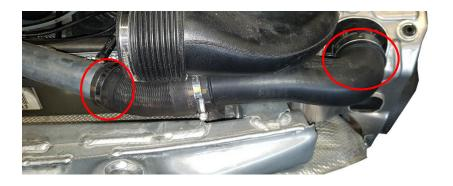
Remove 2x hose clamps, left side breather valve, right side solenoid valve and vacuum line. Then remove the air filter box.
