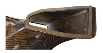
The intercooler consoles on both sides needs to get three small modifications to make space for the do88 intercooler and inlet hoses.
