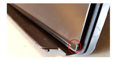
30. On both upper carbon fiber air ducts install the included sealing like this:
