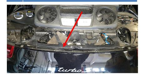
19. Remove the intercooler outlet hose from the intercoolers on both sides by prying out the quick coupling lock clips with a flat screwdriver about 10mm and then pull hose straight out from connection.
