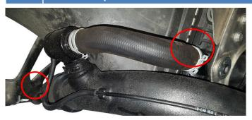
On both sides. Remove 6x C-clips that holds the intercooler in the console.
