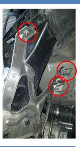
25. On both sides. Remove the turbo inlet pipes, 1x hose clamp on the intercooler outlet tank and 1x C-clip from the console.
