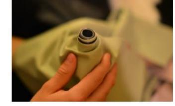
**Step 3:** Turn the boot inside out and insert the knob until the base of the knob is even with the base of the boot. Install rubber O-ring over the boot and align with the grove in the knob.
