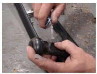
**Step 4:** Pull the knob out of the boot until the O-ring will not allow you to pull any further. Re-install shift boot/knob assembly. Set desired height of the shift knob and tighten the set screws at the base of the knob.
