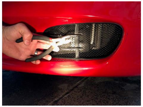
5. For the passenger side, the temperature sensor will need to be removed from its perch, easily pulled out towards the radiator. Once out, insert the grille into the radiator cavity and feed the temperature sensor back through the grill and re-insert the sensor into its perch. Then complete steps 3 and 4 to complete the installation.
