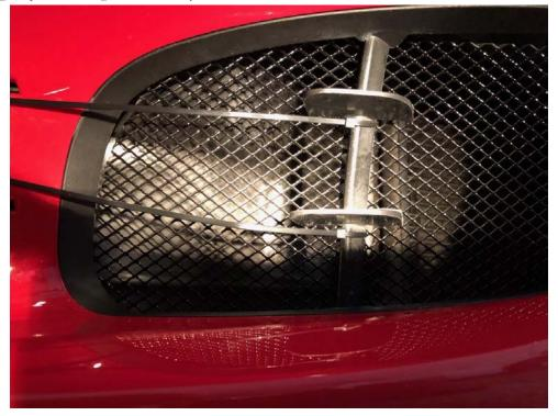
4. Once positioned to ensure no gaps around the edges, pull the cable ties taught and clip off the tails with side cutter pliers.
