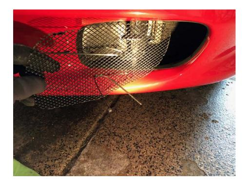
3. Insert gille, position the grille and loosely connect the cable ties under the middle mounts as shown.
