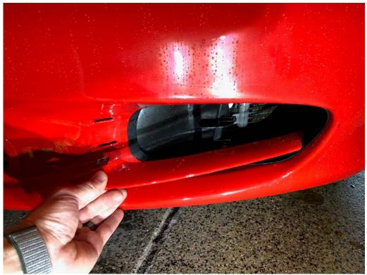
2. Insert the grill as shown, the driver's side does not have a hole in the screen. The passenger side has a hole to accept the temperature sensor.
