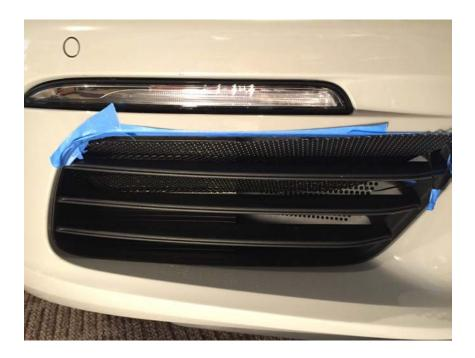
2. Cable ties are preinstalled for ease of installation. Once the grill is inserted, you will be able to rotate the side in your hand into the cavity of the radiator intake. Connect all cable ties, but do not tighten. Once all are connected, rotate the receiver end of the cable tie towards the grill. Once done for all cable ties, tighten by holding the receiver end close to the grill and pull.
