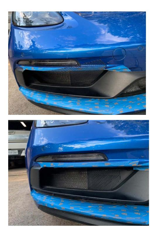
10. Using screwdriver/hooks, slide screen from left to right into grove (shown in the first photo is the right grille, but same concept, slide into the space between the outer bumper cover and the inner air dam):
