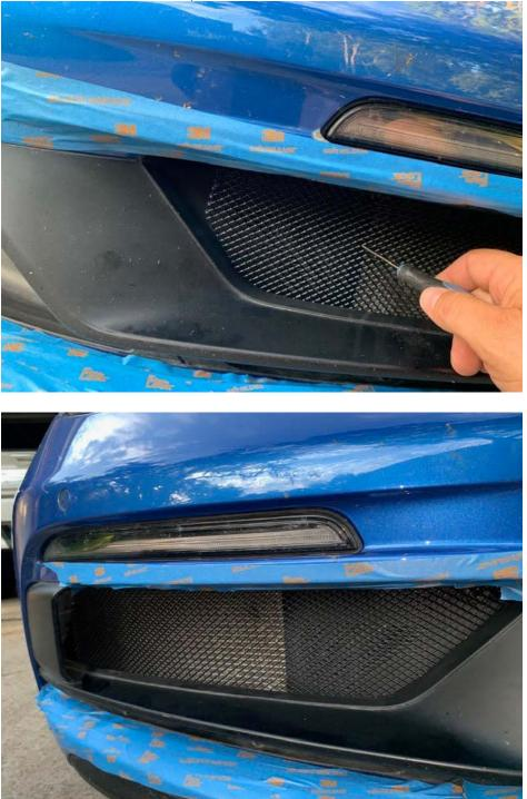
11. Now find the vertical slats below the lower rib and place the cable tie into position. This customer shows the cable tie bent at the tip to be able to do the cable tie installation with out removing and reinstalling the grilles. Each method works.
