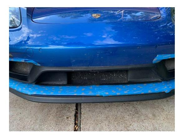
3. Center section - The Bi#ch! Bend center section into concave shape. Don't overdo it. The more you bend it, the easier it is to insert, but the more difficult it is to move it into position.
