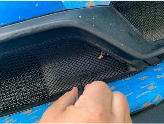
7. Once in position side to side, you need to slowly, patiently, start pulling grill with the tools to pull the concave out of the grill. It takes a long time, slowly pulling at each section. As the grill comes forward, you need to try to push it up into the slot at the top while also getting the bottom rubberized bend under the plastic lip:
