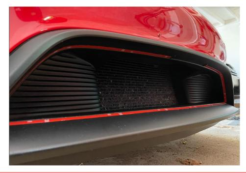
5. Start in the corner and start peeling back the tape backing. Adhere the grille slowly and straightly as possible. Work each inch and press the black trim of the grille into the 3M tape, holding with pressure for a couple seconds. This greatly increases the strength of the connection. Work your way around the opening until complete. You can install cable ties to aid in positioning of the grille as shown below.
