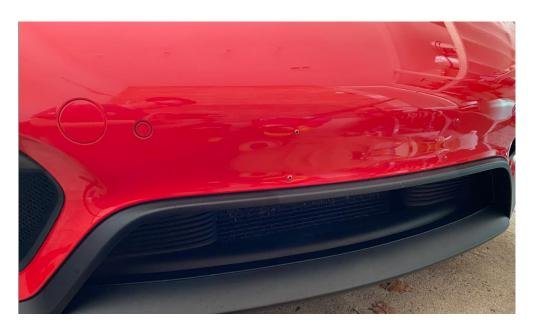
4. Align the 3M tape on the newly cleaned surface as such. License plate brackets need to be removed for installation. Align the circumference with the 3M tape.
