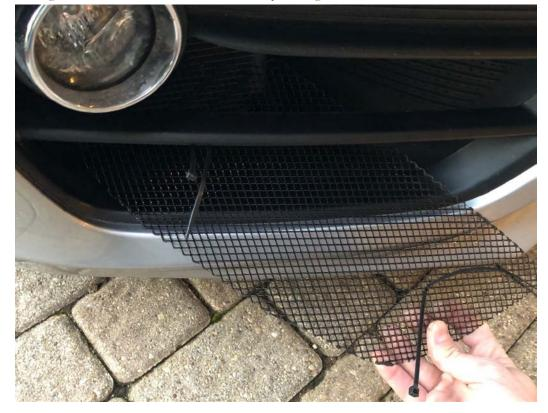
2. Cable ties are preinstalled for ease of installation. Insert hand into space above the middle rib. You will find that using your hand to guide the grill mesh up and to the outside of the car will assist with installation. Do not force the grill. Once the grill is inserted, you will be able to rotate the side in your hand into the cavity of the radiator intake.
