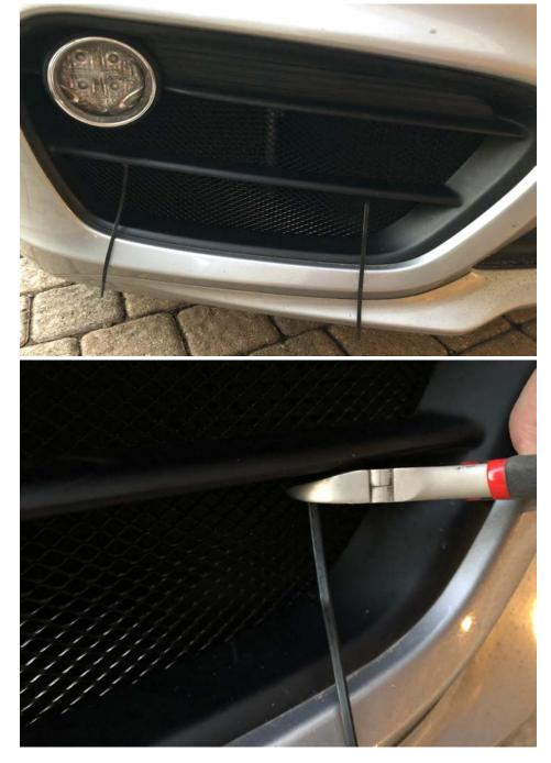
5. Should look like the photo below. Then using a side cutter, clip off the extra cable tie tail.
