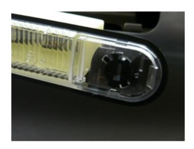
**8.** You are ready to install your new 3<sup>rd</sup> brake light, simply install it in the 3<sup>rd</sup> brake light cut-out, make sure you insert the black tab on the left of your 3<sup>rd</sup> brake light behind the cut-out. Now lock the tab with a screwdriver so that the 3<sup>rd</sup> brake light is secured on the trunk lid, and install your small cover.
