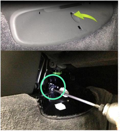
**Step 2:** Then remove the two T-20 torx on both sides, and then pull the two panels towards the back of the car.
