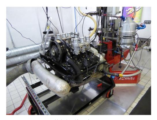
Freshly built and 'run in' 2.4T Motor
