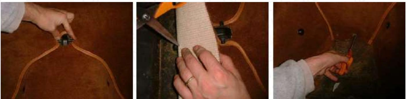
5. Carpet underneath rear seats: mark hole for clips (so that material will be pulled somewhat tightly). Cut small holes with end of scissors and fit clips (picture 5A). Make incisions to fit around the transmission tunnel (picture 5B). Mask the carpet to avoid glue spray over. Glue and press to fit (picture 5C).
