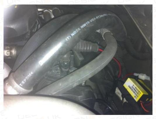
**Step 12:** Run the Red wire into the right hand bank air flow meter wiring rubber boot and solder to RED and BLUE wire (pin 2) of air flow meter harness. (This is an ignition feed and doesn't affect the signal from air flow meter to ECU).
