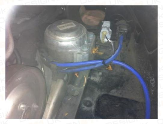
**Step 11:** Take control box and install on right hand side of engine bay onto main engine harness. Run the thin black Ariel wire along loom away from engine.
