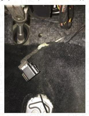
6. From I-Drive box take the piece of loom and connect to throttle pedal connector.
