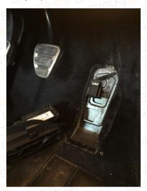
5. Pull carpet forward slightly and re-route pedal connector to appear at top of carpet.
