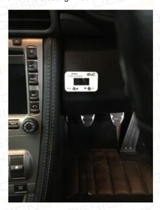
Run the wiring from the unit down behind between the dash and centre console so the small connector appears by the small connector of the loom next to the centre console and foot rest.
