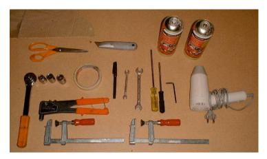
Spray glue for automotive use (2 cans) Scissors Stanley knife Metric ratchets (M13,M15,M17) Riveting tool Lock presses (2) Metric spanners (M8, M10, M13) Ballpoint pen Masking tape Screwdrivers (flat and Phillips) Hairdryer (if necessary)
