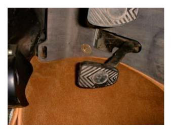
8. Carpet over doorframe (right): Try-fit and mark hole for lower seat belt bolt (picture 8A). Cut hole with end of scissors and fit bolt. With bolt attached, glue and press to fit. Fit aluminium strip (picture 8B).
