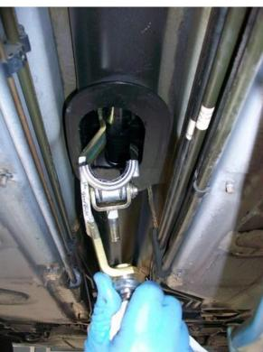
When the shift lever and shuttle half ardraost in place, slip the upper shuttle half in the opposite side of the opening. The goal is to just get it up there at this point.
