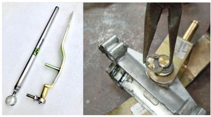
Slide the new shift lever tip into the rubber boot after pulling it down a bit.
