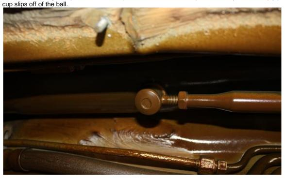
Use a small screw driver to pry e-clip off. There will be 3 washers (2 flat and one wavy washer). The wavy washer is sandwiched between the 2 flat washers and keeps tension on the e-clip and bushings. Slide shift rod and rubber boot out of the way.
