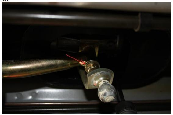
Remove the four 4mm Allen head bolts (See red paint in photo below)
