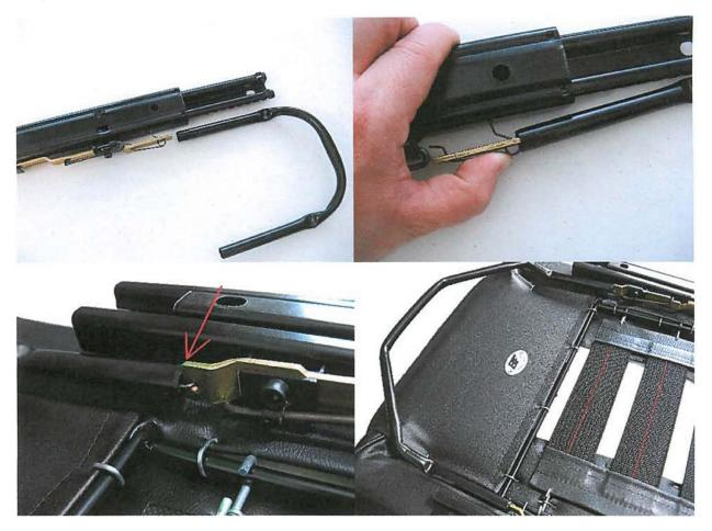
Now insert the adjustment handle on the actuating lugs of the seat reails. Depress the spring slightly as shown in picture. Push the handle onto the lugs as far as it will go.
