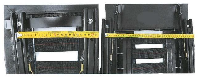
Check the front and rear distance between the bolt centres on rails to ensure they are parallel. There is a little play in the holes to allow for alignment. Set the distance at either 200mm or 385mm and tighten the bolts to lock into place.
