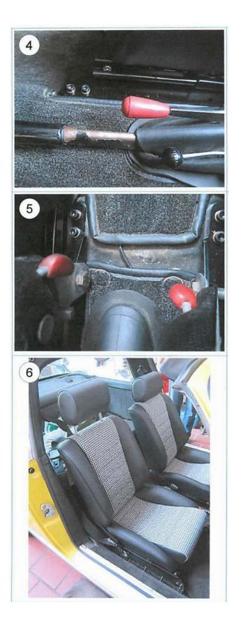
Slide the seat forward and attach rails at rear. Once all bolts are in place, tighten all nuts and check that seat slides forward and back easily and does not bind. If it jams, loosen all 4 nuts and slide back and forward, then retighten.
