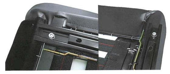
**!!Caution, Insert the bolt and only hand tighten to avoid damage to the thread!!**
