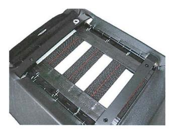
Insert the 5mm thick washer between the seat and seat rail. Start at the front of the seat.
