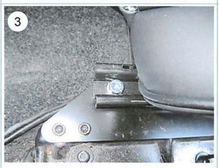
Attach the seats which have the rails already mounted to them. Using the handle, slide the seat all the way back exposing the front attachment holes of the rails. Using M8 x 25 bolts, flat washers and M8 Nyloc nuts, attach the rails to the brackets and tighten the nuts loosely.
