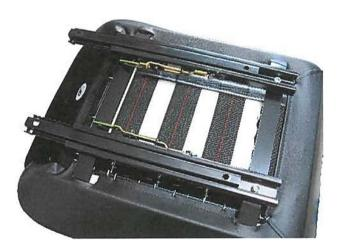
Attach the rail at the rear and hand tighten. Attach the rear rail also.
