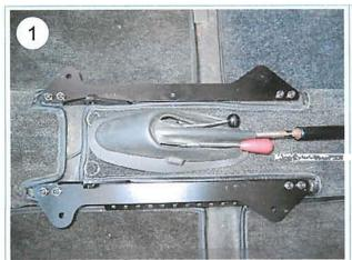
Remove the original seats, including the original seat rails.
