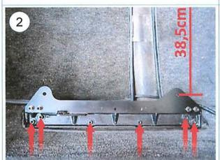
On the outer sills, attach the brackets to the original mounting holes with the seat belt attachment points at the rear also facing outwards. The distance between the hole centres on therese brackets wehre the seat rails attach should be 385mm.
