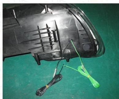
**Step 2:** Please connect the black one to the black wire of the parking function of the light (negative), and connect the green one to the green wire of the parking function of the light (positive).Please do this way for both sides of the light.
