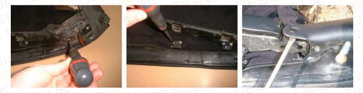
Remove the rubber seals on both sides of your top by taking out the screws in the rubber apertures (picture 2A). Now remove the 2 steel guides left and right (picture 2B). Use a metric spanner (M13) to remove the top guide pins (picture 2C). Your roof skin can now be removed.
