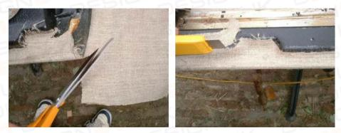
Place the foam backing on top of the linen covering. Spray the edges as indicated by the tape (picture 6A) and press the foam to fit. Use scissors to cut away excess materail along the edges of the frame.
