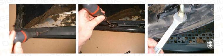
3. Once your roof skin is taken off, the linen and padding can be removed. Your top is now fully dismantled. Inspect the frame for poper operation. In particular, pay attention to the condition and snugness of the tension bands (under thumb on picture) when the tension bars are in their extended position. Correct, clean and paint as required. Do not throw away your old top pieces. 'Reading' your old top may help to install new ones to perfection.
