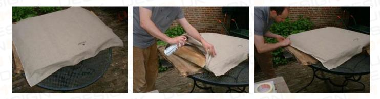
5. Apply spray glue to the inner side of the Targa top frame edges. Cut away corners at 45° (picture 5A). Flod the linen over the edge and press to fit. Use a Stanley knife to cut away excess material (picture 5B).
