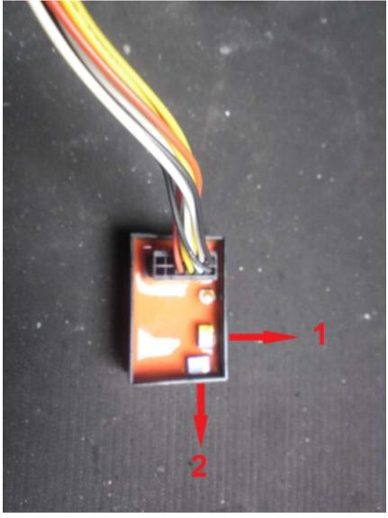
There are two small poteniometers at the torque limiter.
