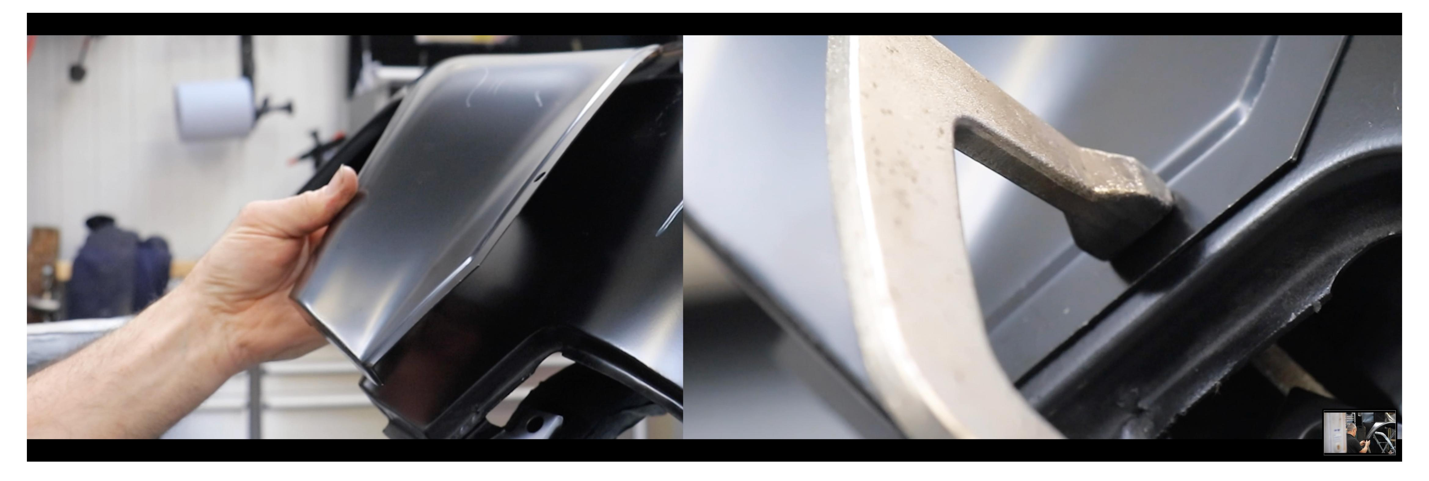
Align the wheel arch so it lines up with the original arch and lower sections.
