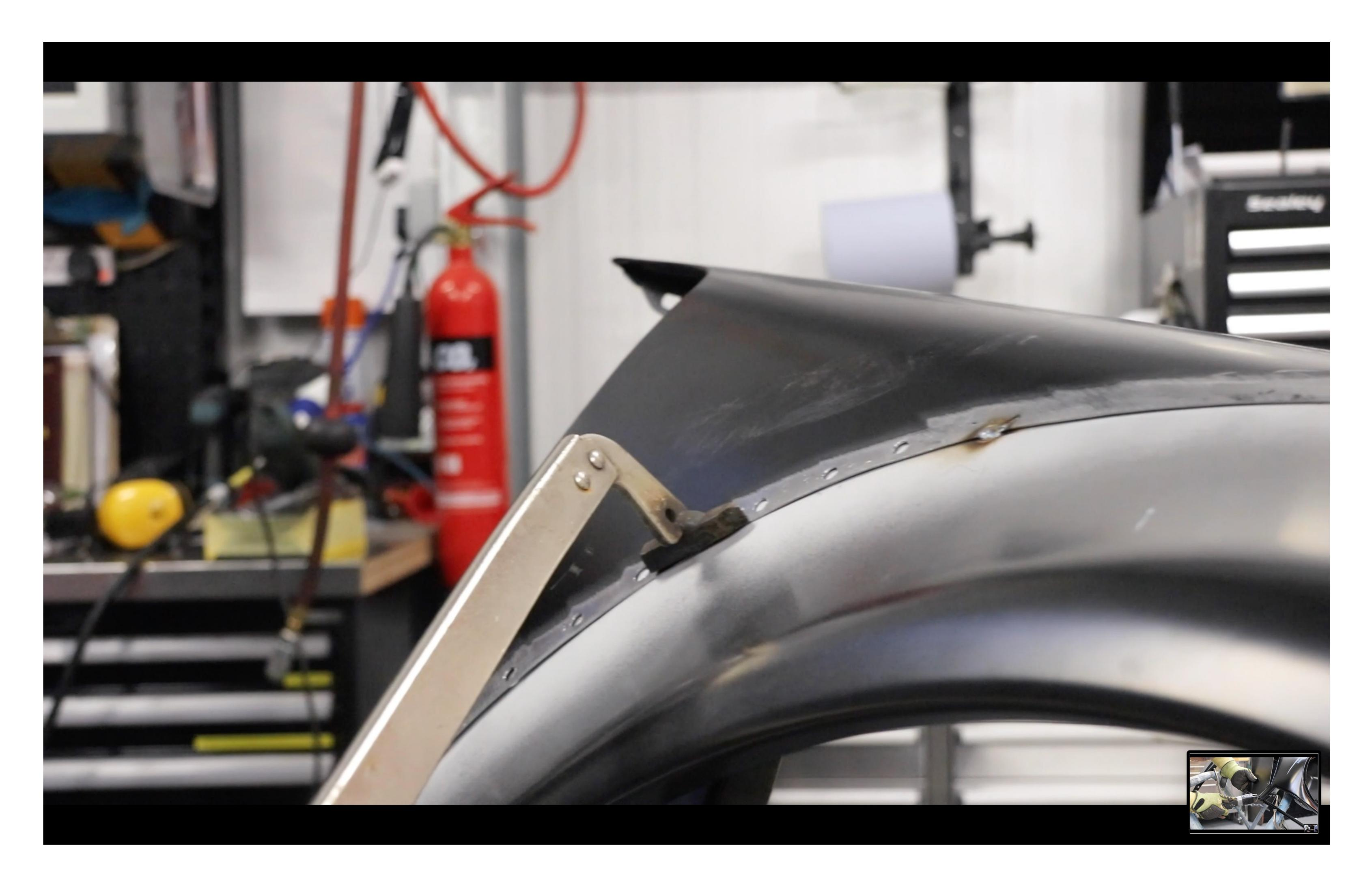
Clamp new arch in place, making sure recess follows the cut line.
