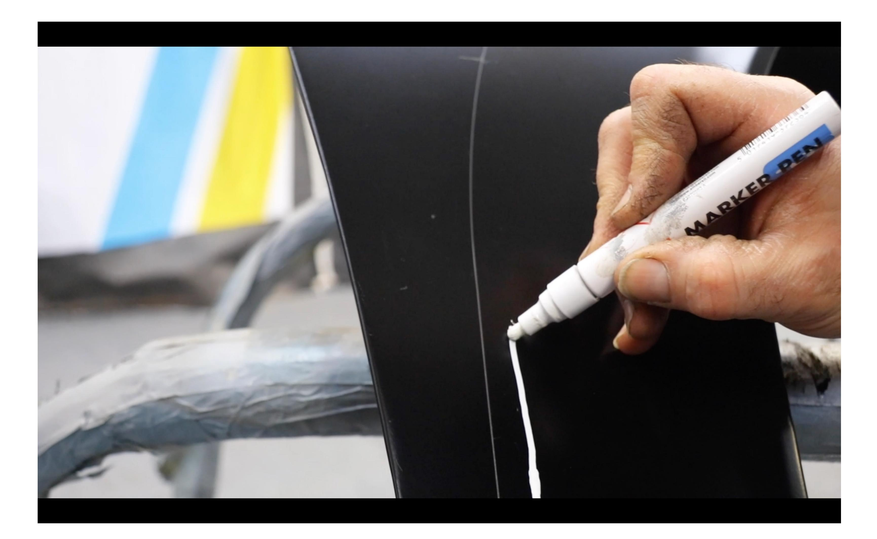
Remove the wheel arch, deduct 3mm from arch measurement and scribe inside previous line.
