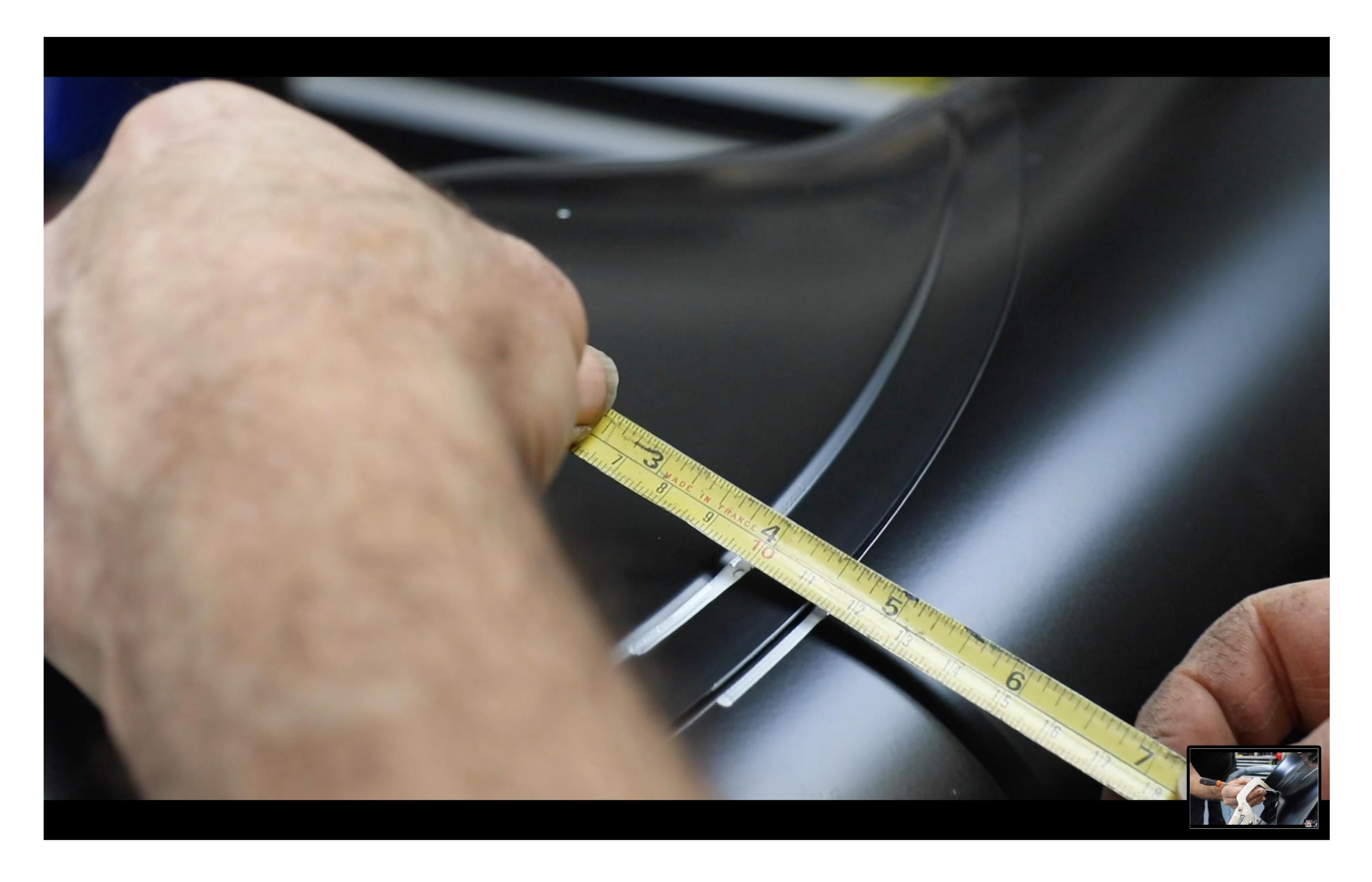
Measure recessed lip on edge of arch, in this case 15mm.
