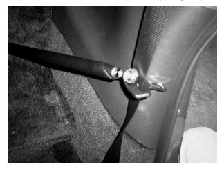
Step 7. Tighten rear seat belt mounting bolts left loose from step 2.
