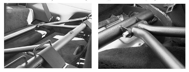
Step 6. Attach rod ends from the support rods (See figure 7) to the harness mount bar using the supplied hardware.
