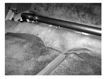
Step 5.Attach the harness-mounting bar to the rear-mounting bar with the supplied hardware as shown. (See figures 5 & 6)
