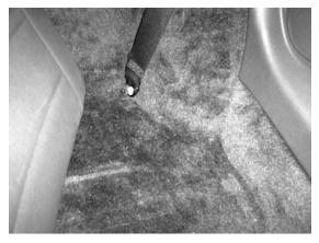
Step 2. Remove both outside rear seat belt mounting bolts and hardware. Position support rods and reinstall seat belt and mounting hardware just the same as it came off. Do not tighten at this time. (See figure 2)
