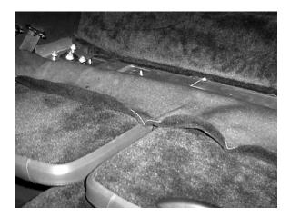
Step.4 Remove the (3) strut mounting nuts on each side. Position the rear-mounting bar as shown. (See figure 4) Reinstall nuts and torque to factory specs. Reposition carpet.
