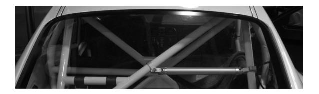
Step 4: Reference belt harnesses manufacturer's installation instructions for mounted the shoulder harnesses to the R-1040. It is common practice to cross shoulder belts to prevent slippage. Use collar clamp to separate belts and avoid overlapping.
