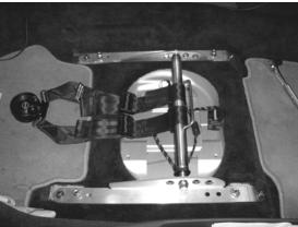
The sub-bar length is adjustable, and includes two pivot washers for each side to prevent preload on the floor mounts when the bar is tightened. This will allow the floor mounts to stay true during reinstallation after the seat is mounted. Half inch open ended wrench should be used on the adjuster to bring flush and hold as the flange head bolts are tightened. The rounded side of the pivot washer will seat in the machined radius chamfer. Avoid preload on the floor mounts. Tighten Jam Nut.
