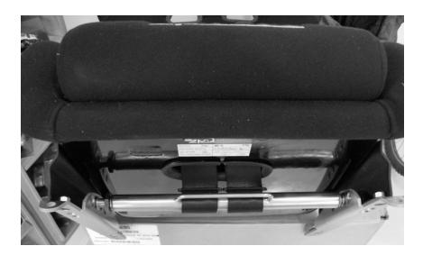
Step 5. Reinstall the seat assembly in the car with the stock E-12 Torx bolts. A E-12 wrench will be needed to tighten the rear bolts if the furthest back position is used (the rear most mounting hole on the R-907X bracket will be positioned over the rear floor pan bolts.
