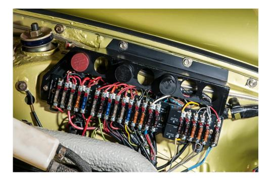
Note: The original lid will fit over the new panel but the recess on the far right hand end may need enlarging but a few mm for a good fit.
