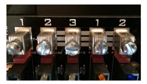
Note1 : Late model cars may have extra 'intermediate' terminals fitted in between the numbered terminals. These wires can be fitted to either adjacent terminal on the new panel. For example, if you find a wire on a terminal between 7 and 8 on the old fuse block, then wire it to 7 **or** 8 on the new panel.
