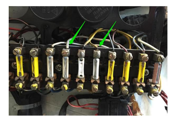
The M062 control unit sends a signal on the yellow/black wire that can cause the relay to buzz on 911-FPR fuse panels up to and including versions 1.2. If you have this option, please disconnect the yellow/black wire (tape up the end)
