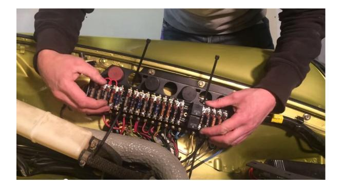
6. Starting at the left hand end (rear of car), transfer each wire from the original screw terminal to the new one until you have completed the bottom row. Note that in many cases there are multiple wires in the same terminal. It is vital that you are methodical and take your time. Complete each terminal fully before moving to the next one. Skip the 'H'
