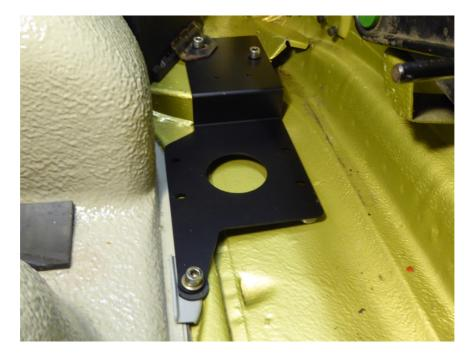
Out of the car, attach the plate to the bottom of the compressor. Also attach the relay bracket to the plate. The assembled unit can now be placed in the car.
