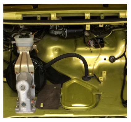
With old blower removed, identify holes for cabin wiring and wire sense lines to high power accessory switches.
