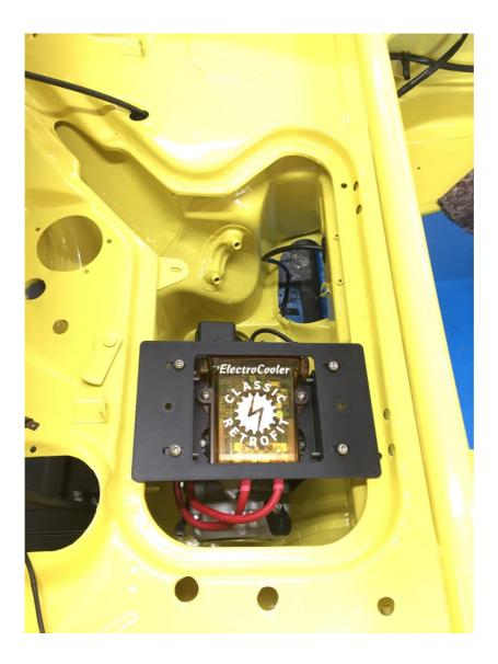
The clamps are used to secure the compressor cradle. It is probably best to do the final clamp down after the hoses have been fitted (as you may want to lift the compressor to attach the fittings).
