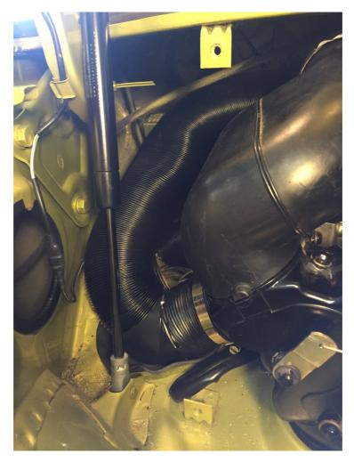
'T' piece in place (bottom of picture) with branch running to inlet of new blower.
