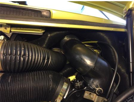
Pushed under the scuttle, the 60mm recirculation duct runs between the 'T' and blower inlet.
