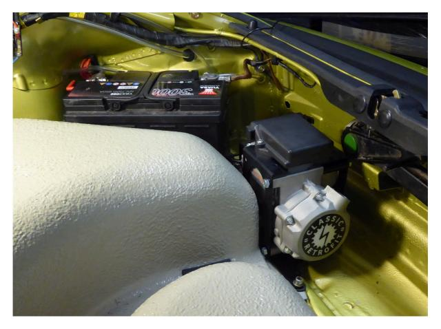
Insert the 3 M8 bolts using the washers provided. The thick black wire from the compressor MUST be attached to the forward bolt.
