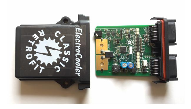
The ECU comes preset with typical working parameters for a 911. It is possible to adjust the values using a laptop as described in our setup manual. It is strongly recommended NOT to adjust these values without consulting us first.
