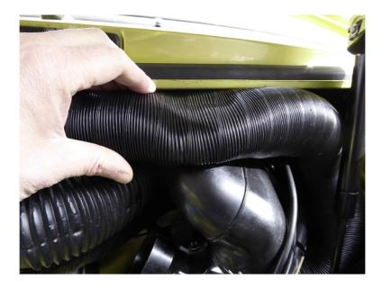
On cars with centre vents, on passenger side the duct must route over the screen duct. Gently squash the duct and push it up under the scuttle area. This is a RHD car. On a LHD, the squashed tube will be on the left hand side
