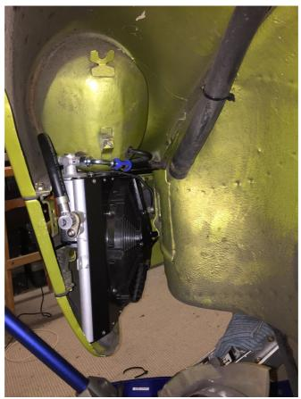
Condenser and fan assembly fitted. It's tight!
