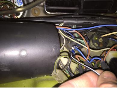
Attaching a 'piggy back' sense wire to the rear defogger switch. This tells the A/C to cut back on power if this is switched on.
