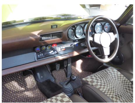
Discrete control button placed in blank to the right of heater sliders. The ring led indicates A/C status.
