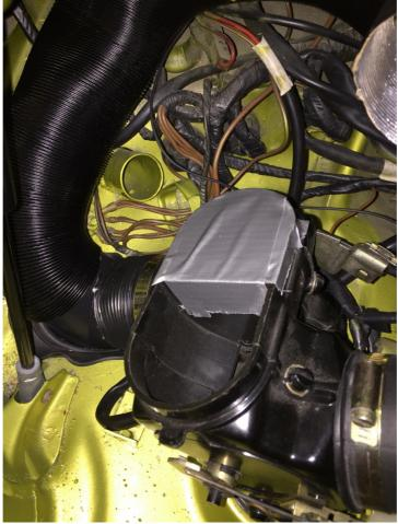
left of picture, the 'T' piece sitting in the bulkhead gasket with 60mm branch heading upwards.
