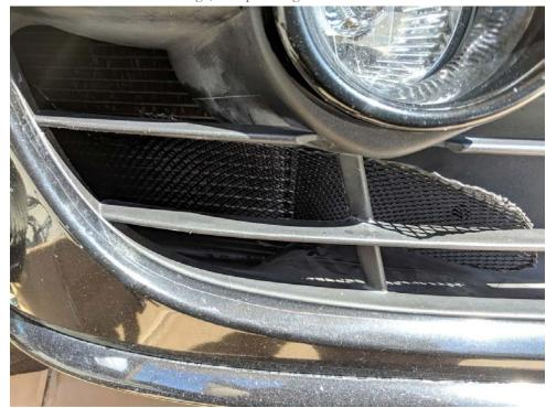
6. The little tab of material which would flanks the fog light will need some more bending to clear OEM plastic as the grill is pulled towards the center. It is easily bent back to the original shape.
