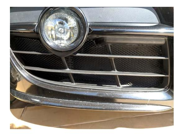
7. Use a hook or other tool to fine tune the position and pull the grill towards the front of the opening so that it will be flush.
