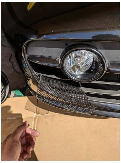
3. As the grill is fed through, it should be guided down towards the bottom of the radiator. Having smaller hands help here because you can reach in through the adjacent vent opening. Bending upwards may also provide more room to insert the grill fully.
