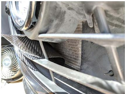
5. Once the last corner is fed through, then pull the grill towards the center of the car
