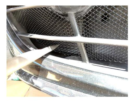
8. Connect the cable ties loosely and snug them as you push the receiving end towards the grill material. This ensures that the receiving end, when tightened is as hidden as possible. Secure the cable ties and snip off the tail ends.
